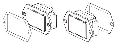
Secure BDI with M 2.5 bolts or screws.
