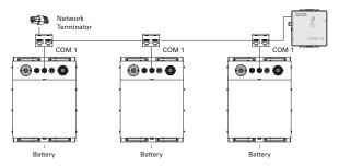
Figure 3. AEbus Network Termination
