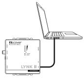
Figure 7. Configuring LYNK II with LYNK ACCESS software
