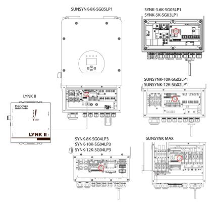
Figure 6. SUNSYNK CANopen Connection
