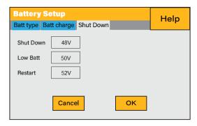
Figure 11. Battery Shutdown Settings
