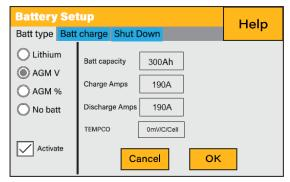
Figure 9. Battery Setup for 3 x AES RACKMOUNT Battery Modules
