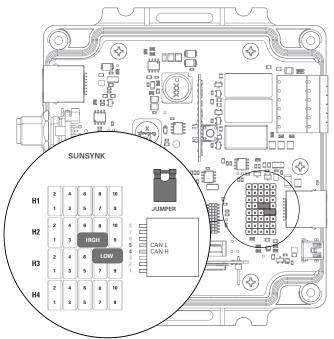
Figure 2. CAN pin assignment for SUNSYNK communication
