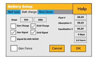
Figure 10. Battery Charge Settings for AES RACKMOUNT
