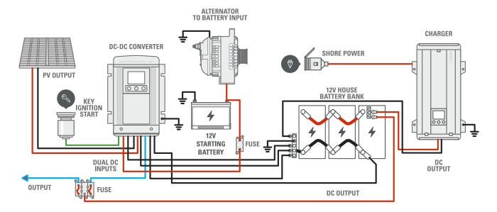
The above schematic should be used only as a guide. Ensure the installation of your system meets local code requirements and seek the help of a certified professional.
