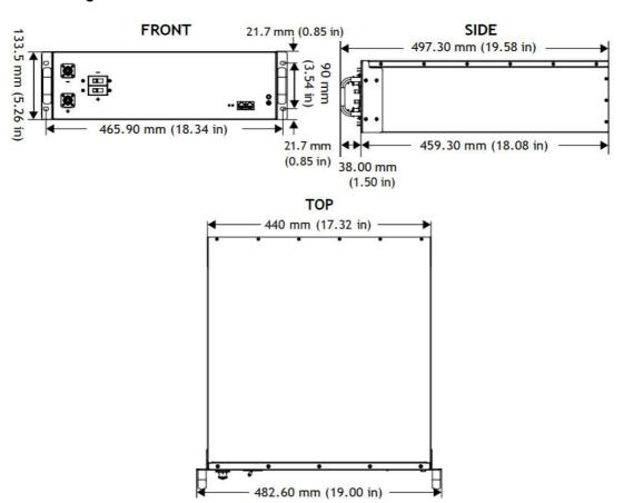
Figure 1. Diagram with overall dimension (Unit: mm)
