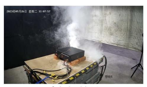
Smoke release during test
