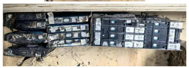
Damage of the internal components
