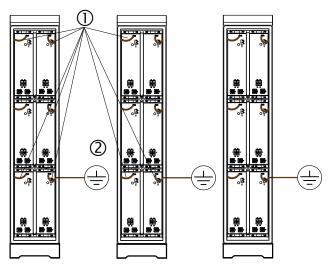
Figure 2. Grounding Example: Slimline Enclosures
