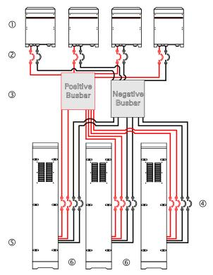
Figure 1. Wiring Example: Slimline Enclosures
