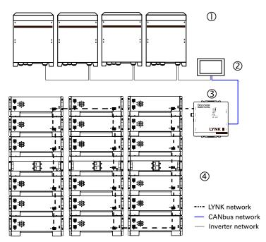
Figure 6. Communication Example: LYNK II and Battery Modules in Quick Stack Racks
