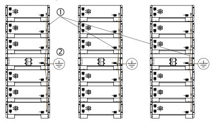
Figure 5. Grounding Example: Quick Stack Racks
