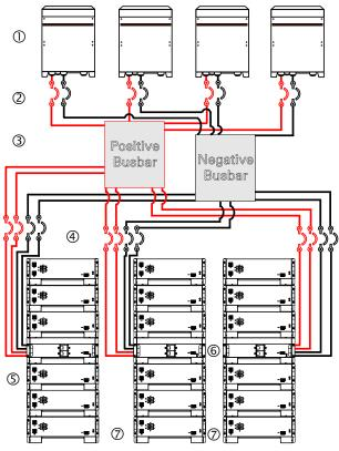
Figure 4. Wiring Example: Quick Stack Racks
