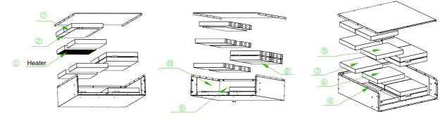
Remark: The number 1~10 means Thermocouple no. T1~T10 distributed in modules.
