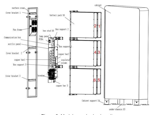
Figure 2. Module numbering in unit
