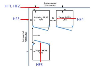
Figure 11. Heat flux sensor layout
