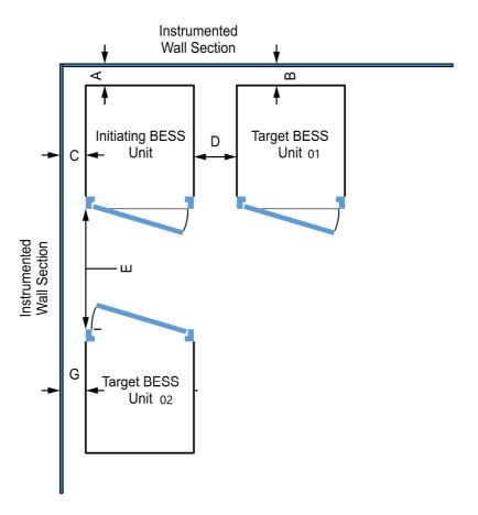
Figure 1. Top view of sub-unit's layout
