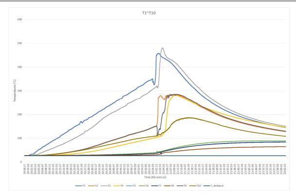
Figure 8. Temperature vs time curve of module 04 in initiating unit.
